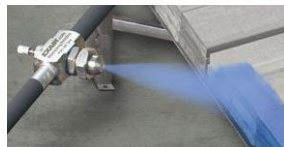
A Model AN1010SS Internal Mix Narrow Angle Round Atomizing Nozzle is used to mark strips of steel before they leave the mill.
