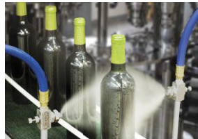
(2) Model EB1030SS atomizing nozzles are used to give a final sanitizing rinse prior to labeling wine bottles.
